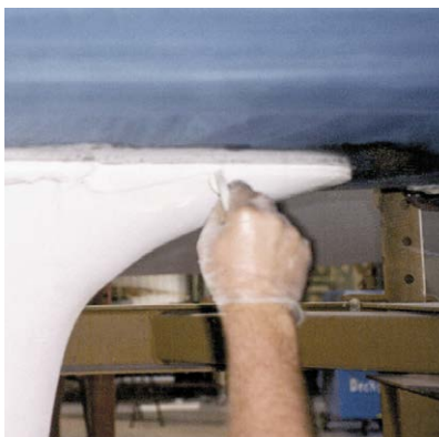
Fig. 13 The joint is tooled off and finished
